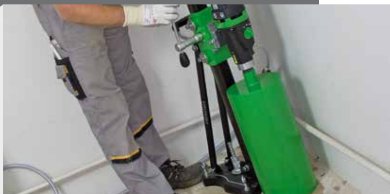
BST 182 V/S: mounted carriage on 4 special balls
